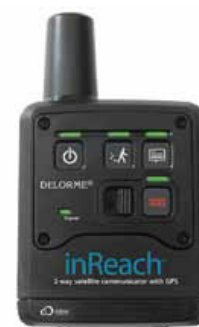
Both the DeLorme inReach (above) and the Iridium 9675 Extreme use the new Iridium 9602 modem, which allows two-way communication. The recently introduced 9675 was recalled because of antenna problems; Iridium says the problem has now fixed.
